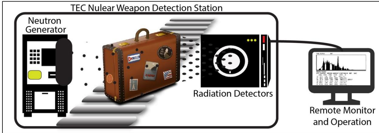
*When suspected material is bombarded by low energy thermal neutrons (produced by the Hadron neutron generator), the nuclei of the fissile materials are split into smaller, more stable isotopes, and various radiations are released. This increase in neutrons is immediately detected by various detectors which monitor and record the anomalies. Whenever a spike in neutrons is identified by the computer software, the suspected container can be flagged for further examination by DHS/TSA authorities.*
